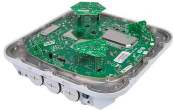
RUCKUS BeamFlex® Smart Adaptive Antenna
